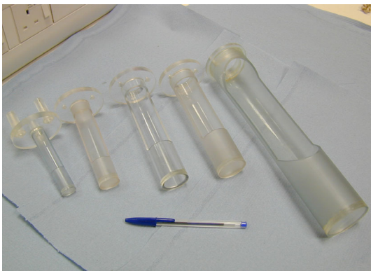
Fig. 1. Polycarbonate detachable cradles for 20, 28, 35, 40 and 60 mm nominal diameter RF probes.
