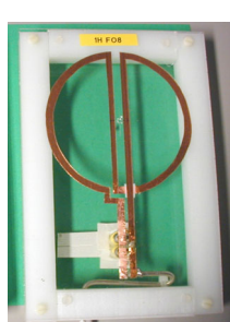
Figure 1. Circular figure-of-eight (FO8) surface coil (2R=10 cm, 2s=1 cm) 1.5 T prototype.
