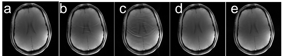
Fig. 3: Full-FOV acquired image a) and GRAPPA reconstructed PPA2 b) PPA3 c), MCMLI reconstructed PPA2 d) and PPA3 e) images.
