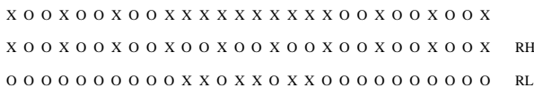
Fig. 1. Top: 28 samples of a variable density ky data set with threefold undersampling and eight Nyquist-sampled center points. Center: high resolution component RH , Bottom: low resolution component RL . X and 0 represent measured and unmeasured points respectively.
