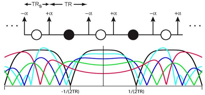
**Figure 1:** (top) wbSSFP pulse sequence and (bottom) signal profiles during TR for  $TR_s = \{TR, 0.8TR, 0.6TR, 0.4TR, \text{ and } 0.2TR\}$  in {black, cyan, blue, green, and red}. Profiles assume  $T_1 = T_2 \gg TR$  and  $\alpha = 90^\circ$ .
