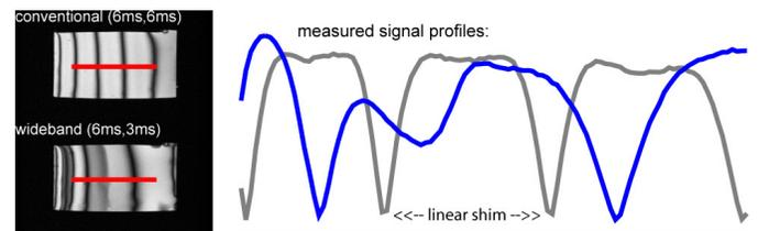
**Figure 3:** Measured signal profiles from a uniform block phantom with a linear x-shim at 1.5T, with  $TR = 6$  ms: (gray) conventional SSFP with  $TR_s = TR$ , and (blue) wbSSFP with  $TR_s = TR/2$ . 60% bandwidth improvement is observed. The signal dip in the wbSSFP profile is presumably due to the test object.
