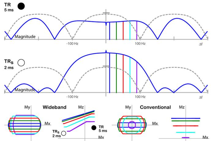
**Figure 2:** Illustration of steady-state for  $TR_s = 2$  ms and  $TR = 5$  ms. (top) signal profiles during TR and  $TR_s$ , and (bottom) magnetization path compared with conventional SSFP where  $TR_s = 5$  ms. Simulations assume  $T_1/T_2 = 1000/300$  ms and  $\alpha = 70^\circ$ .
