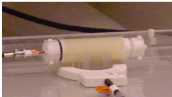
Fig. 1: Cylindrical shaped phantom filled with gel containing a dipole constructed from a semi rigid coaxial cable. Left: photograph of the phantom and the 3-inch coil. Right: dipole dimensions showing inner, outer and insulator dimensions. Middle: illustration of the phantom.
