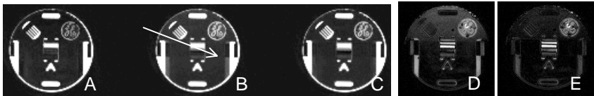
Figure 1. Phantom data collected using a 3D breast protocol. (A) full kz data (B) image from truncated kz (C) predicted image from truncated data. A,B,C are on the same windowing scale. (D) subtraction image of truncated data image from original image. (E) subtraction image of predicted image from original image. E,D are windowed on the same scale.
