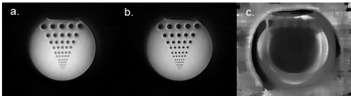
Fig 1. Spiral images of a resolution phantom: a. uncorrected image, b. deblurred image, c. calculated fieldmap showing optimal offset reconstruction frequency.
