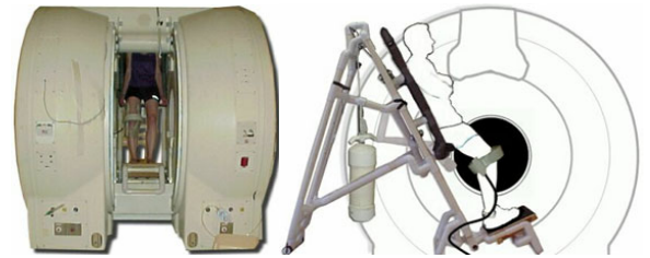
Figure 1: Backrest placed inside the SP magnet.
