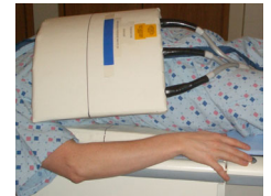
Fig.1: Positioning of the rigid 32-element coil used in the volunteer study (21-element coil segment is placed on top)
