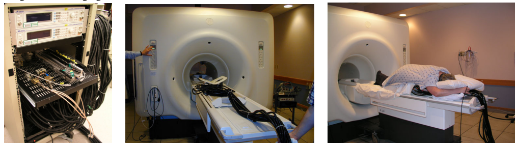
Figure 1. Photographs of the source-detection system are shown at far left, and in the middle the fiber optic array coupled into the breast coil are shown. In the far right, a patient is positioned on the breast coil with fiber array in place for simultaneous MRI-NIR imaging.
