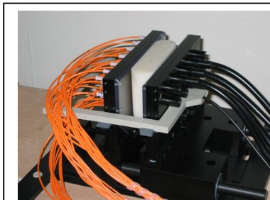
Fig. 1: Compression unit with breast phantom. Illumination fibers enter from the left, transmitted light is collected by fiber bundles on the right hand side. The surrounding surface coil produces a vertical B_1 , allowing the whole block to be rotated around that axis.
