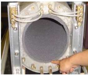
Figure 1. The gradient insert with the absorptive foam
