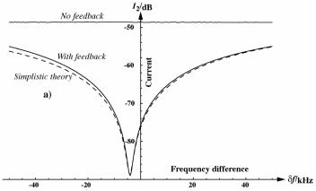
**The reduction in induced current** (in dBs) in the second surface coil with the application of Cartesian feedback as a function of frequency off resonance. Coupling is from a driven first coil via the intermediary of a conducting phantom. (The frequency offset is due to a discrepancy between the spectrometer's and the network analyser's frequency sources.)
