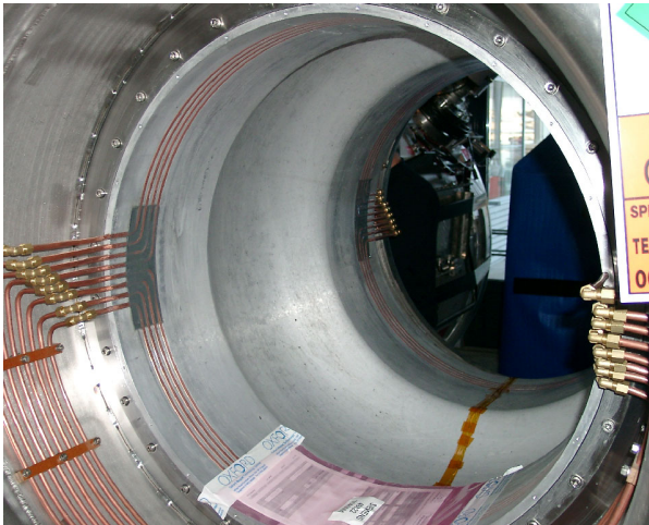
fig. 1: the bulged magnet bore tube
