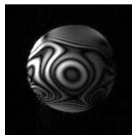
Fig. 4: Transmission with all four channels shows a homogeneous transmit profile. The receiving channel was placed on the left side. A 10\pi -pre pulse was used to acquire a qualitative B_1 -map. This means that there are 10% variation between two black stripes. The used phantom was a 6 g/l NaCl-solution (84 mm diameter) placed in the center of the array.
