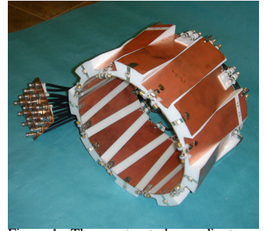
Figure 1: The constructed z-gradient TEM coil
