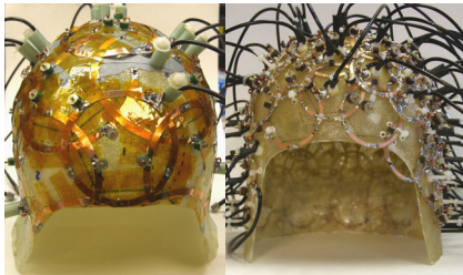
Fig 2 Photo of the 23 channel and 90 channel coil. Fig. 3 noise correlation matrix for the 23 and 90 channel arrays. Fig 4 MPRAGE from the 90 channel coil.
