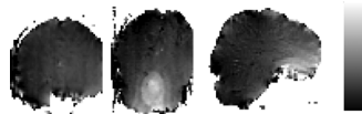
Fig. 2 Change in frequency map (Hz) due to a rotation of 1.7 degrees about the lateral axis.
