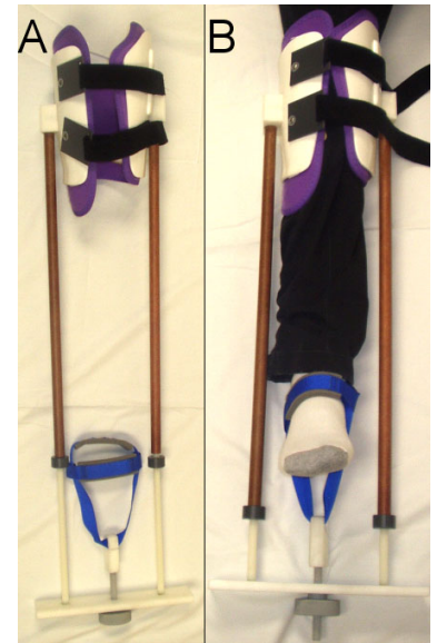
Figure 1: MR compatible ankle distraction device. (A) Construction. (B) In use.
