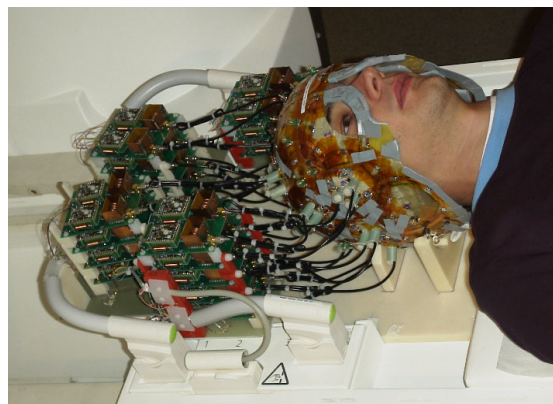
Fig.1: 32-Channel-Head-Coil (without cover)
