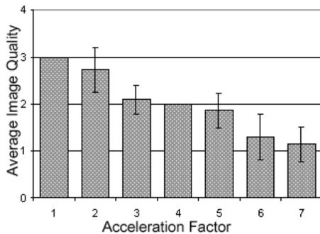
**Figure 2:** Average image quality rating for nonTSENSE data (R=1) and increasing R (2-7).
