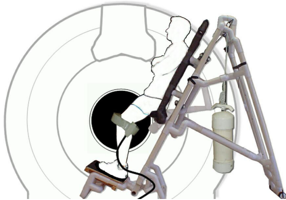
Figure 1: Schematic drawing of our custom MR-compatible back support. The support is made of plastic pipes, a sliding mesh table, and a counter-weight that fits between the two halves of the "double doughnut" GE Signa SP system. The knee is positioned at isocenter.
