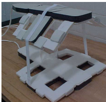
Fig. 1 The DAQD 3D SENSE coil. Fig. 2. Schematic for the anterior four coil elements.
