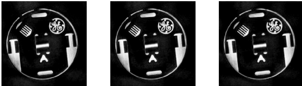
Figure 2: Sample slices from a 256 \times 256 \times 12 voxel data set reconstructed with the modified BURS algorithm using pre-computed interpolation coefficients. The image on the left uses a neighborhood size of \delta k = 2 , the center image has neighborhood size \delta k = 4 , and the image on the right uses \delta k = 6 . Each image set required 2 minutes to reconstruct using the stored interpolation data. As can be seen, all three images show very good image quality from this high signal-to-noise ratio data
