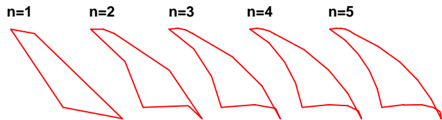
Figure 1. Different segmentations of a coil, which shape is part of a sphere with azimuth opening of 60°, elevation opening of 45° and four sides connected with great circle lines. Calculation showed that n \geq 3 provided enough accuracy.
