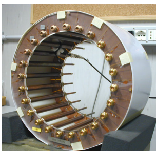
Fig. 2 The 3 Tesla TEM prototype made of 24 coaxial elements.
