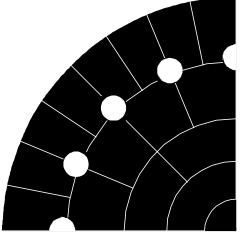
Fig. 2b. Outside Cu foil on one guarter of endcap.
