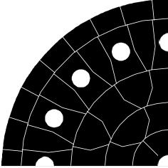
Fig. 2a. Inside Cu foil on one guarter of endcap.
