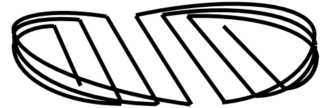
Figure 1: Gradiometer receiver coil design.
