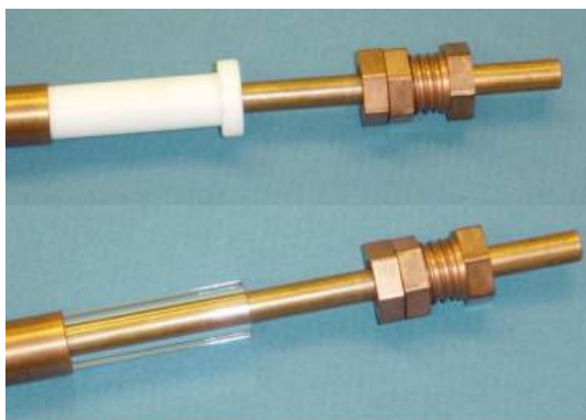
Figure 1: Exploded view of individual elements from the TEM coil showing placement of the Teflon (upper) and quartz (lower) dielectric.
