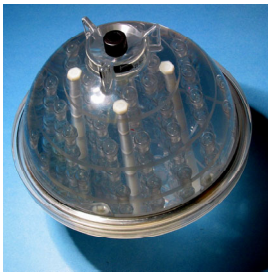
Figure 1: Photo of calibration phantom consisting of 171 small spheres arranged in an array.
