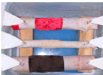
Fig.1: upper view of the phantom showing the 3 bundles: rayon (up), cotton (middle), mercerised cotton (down)
