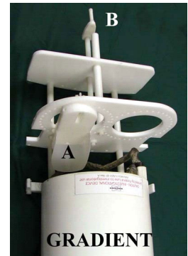
Figure 1: Knee gradient and leg holder. (A) Foot holder can be rotated in 5° increments. (B) Screw adjustment controls position along the z-axis
