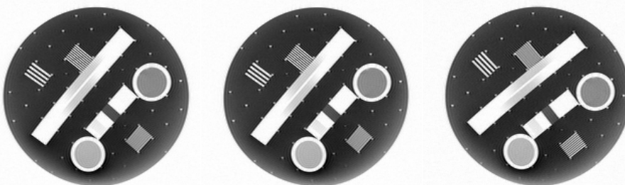
Figure 2: Left the original and middle the motion compensated image by updating the MRI gradients with the data of the tracking system. On the right side no motion correction is activated in the MR scanner. The 10 degree motion is clearly visible. The negatives of the MR images are used.
