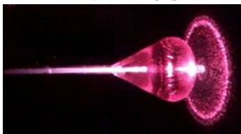
Figure 1 CardioFocus Inc. (Norton, MA) prototype MRI-Compatible laser-balloon ablation catheter inflated, and with laser directed towards distal end. The catheter has multiple lumens, including one for balloon dilation, using pressured D 2 O (dark in MRI and thus a good passive marker), and one providing an optical endoscopy channel, allowing visualization of the vein interiors and thus also improving localization. Laser-ablation is a desired ablation technique, because fiber-optic delivery of light does not cause RF interference or heating. A guiding sheath was not MRI-compatible, and therefore was distanced from the ablation region.
