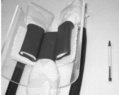
Fig.1: Coil array consisting of three single coils placed parallel to each other. Each coil was wrapped with foam and shrinkable tubing. The coil configuration was fixed on an arced plate of 200 mm diameter made of Plexiglas. The loop dimension of each coil element is 35 x 70 mm. In comparison to the setup a regular pen.
