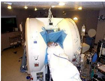
Fig. 1 Positioning of neurosurgical patients in the interventional 0.5 T MRI scanner (GE Signa SP/i).
