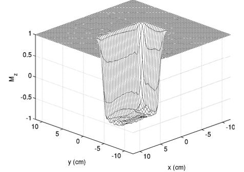
Figure 2. Inversion pattern excited by the fast optimal control-designed pulses, NRMSE = 0.0918.
