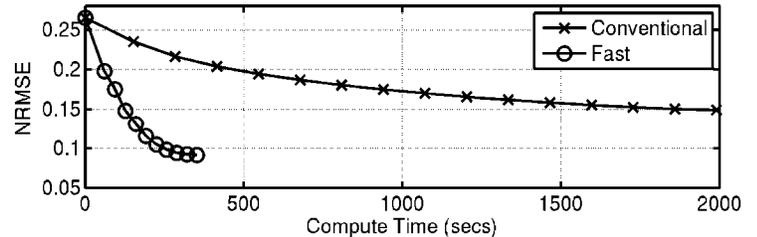
Figure 3. Measured design times for conventional and fast optimal control methods. The fast method achieves a 37-fold reduction in compute time.
