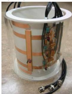
Fig.2. Four channel array for 0.5T
