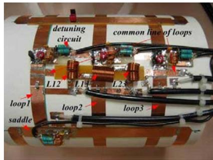
Fig.3. Decoupling circuits
