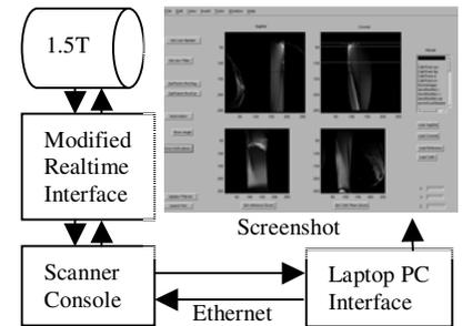
**Fig 2:** System architecture
