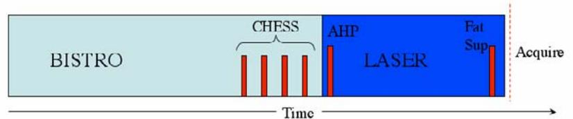
**Figure 1.** Block diagram of pulse sequence. BISTRO outer volume suppression is interleaved with CHES water suppression prior to excitation. Fat suppression is applied after LASER.
