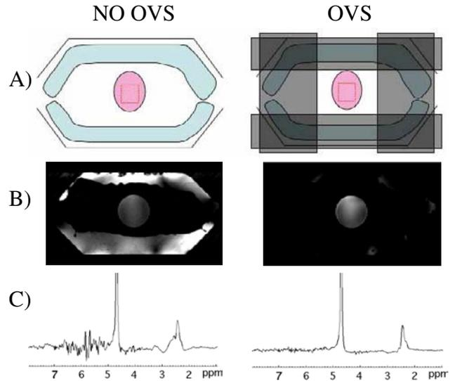
**Figure 2.** Results of BISTRO outer volume suppression. A) Cross sectional schematic of coil showing position of phantom and suppression slabs. B) Flash images with and without OVS. FOV=25x45 cm. TE=11ms. TR=5ms. Matrix= 128x128. C) LASER spectra (8cc voxel) with and without OVS. TE/TR=75/3200ms.
