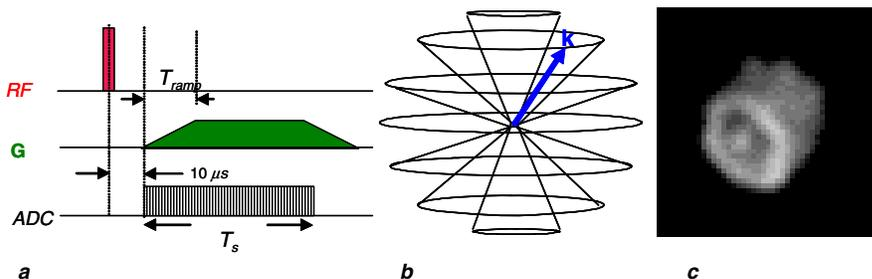
Fig.1 a) 3D radial projection imaging sequence using ramp sampling. b) Sampling on concentric cones for uniform mapping of  $k$ -space. c) Volume rendered image of one of the specimens obtained by 3D radial imaging.
