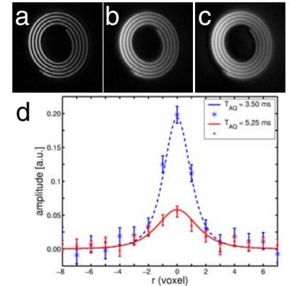
Figure 3: Phantom measurements and extracted blurring function. (a) Short- $T_2$  phantom ( $T_2 = 660 \mu$ s) acquired with  $T_{AQ} = 0.68$  ms. (b)  $T_{AQ} = 3.50$  ms. (c)  $T_{AQ} = 5.25$  ms. (d) Blurring functions (asterisks, dots) obtained from a deconvolution of image (a) from (b) and (c), respectively. The curves represent the simulated decay functions for the respective  $T_{AQ}/T_2$  ratios.
