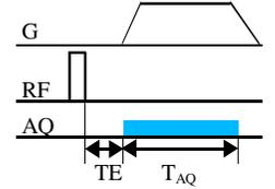
Figure 1: 3D ultrashort TE sequence applying a non-selective excitation pulse and FID sampling.
