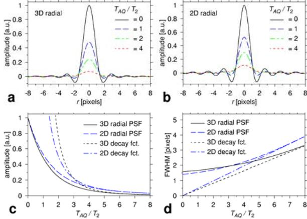
Figure 2: Radial PSF under the influence of  $T_2$  decay. (a) Total PSF in case of 3D FID sampling for different ratios  $T_{AQ}/T_2$ . (b) Total PSF for 2D FID sampling. (c) Amplitude dependence of total PSFs and decay functions (cf. text) on  $T_{AQ}/T_2$ . (d) Linewidth dependence on  $T_{AQ}/T_2$ .
