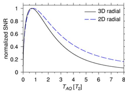
Figure 4: Single voxel SNR obtained from the PSF amplitude (cf. Fig. 2(c)) weighted with the square-root of the sampling window duration  $T_{AQ}$ . The functions have a maximum at  $T_{AQ} = 0.69 T_2$  for 3D and  $0.81 T_2$  for 2D sampling.
