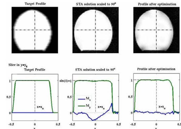
**Figure 1:** Simulation for a  $90^\circ$  3D excitation. *Top row:* Transverse slices in  $z=0$ . *Bottom row:* Slice profiles along  $x$  in  $z=0$  and  $y=y_0$ . Desired uniform magnetisation (Target profile). Predicted magnetisation by Bloch simulation from the parallel transmission model in the STA regime. Magnetisation from the Bloch optimisation. Note the phase profile improvement across the FOV.
