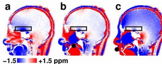
▲ **Figure 2**  $B_0$  maps for comparison of shimming effectiveness. The shim coil locations are marked by black dots.
