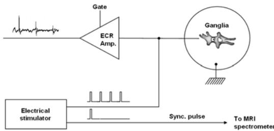
Fig. 1. A schematic diagram of the ECR with electrical stimulations
