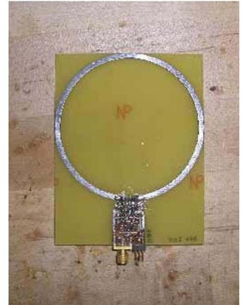
**Figure 1** Untuned coil with integrated amplifier.
