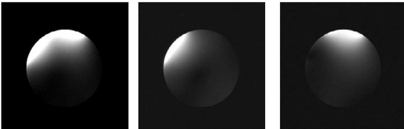
**Figure 2** Phantom images taken with two untuned coils used in an array. Left: combined image; middle, right: uncombined images.
