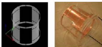
Figure 1 Coil geometries for simulation model (left) and the real coil (right) (Diameter: 50 cm)
