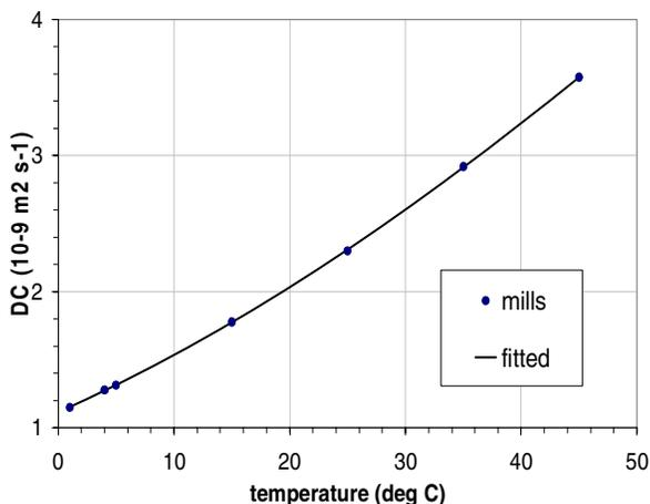
figure 1: DC of water (interpolated from Mills<sup>1</sup>)
