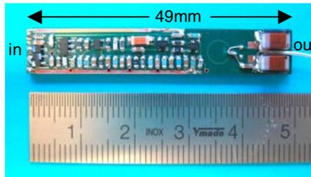
Fig. 2: Lab demonstrator of the feedback amplifier in SMD technology
