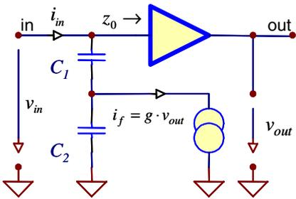
Fig. 1: Basic arrangement of the feedback amplifier
