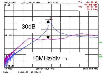
Fig. 3: Wide band decoupling of an MR-loop when the amplifier is switched on
